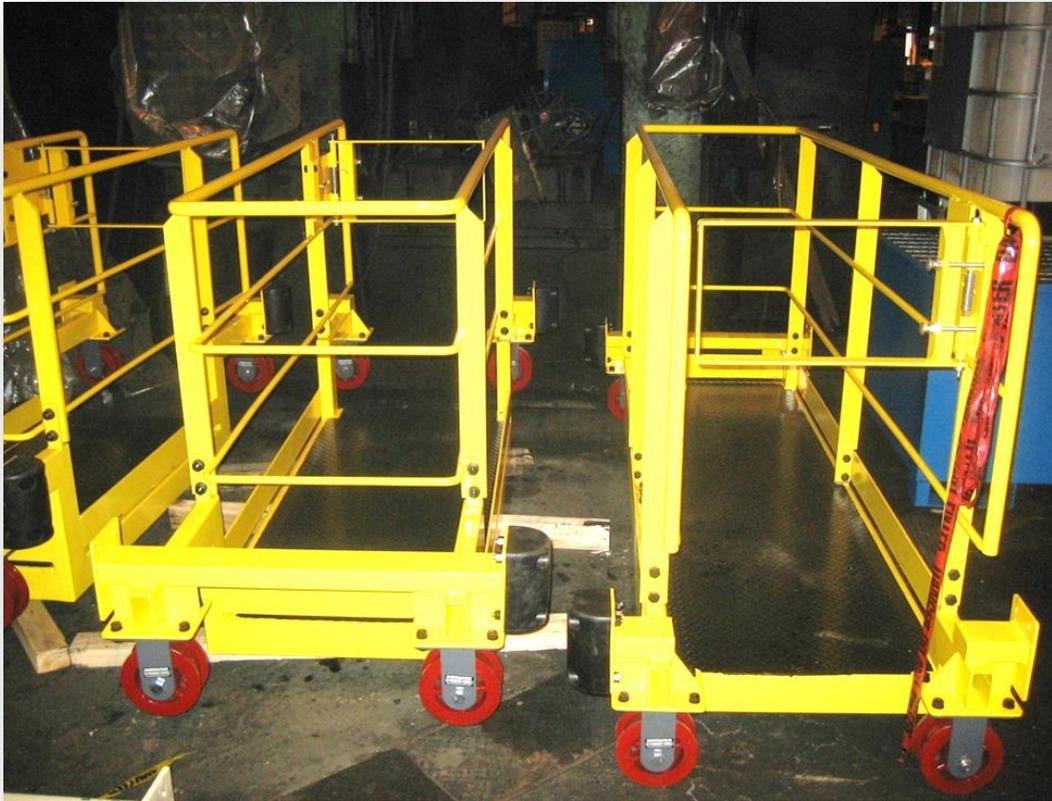
**Problem:** As high bay lights burnt out, maintenance was required to replace them to provide adequate area lighting. Machinery and other obstructions on the mill floor would not allow proper access to the lights via aerial manlifts. Workers would then climb onto overhead crane trolleys with limited fall protection creating a potential fall hazard.
